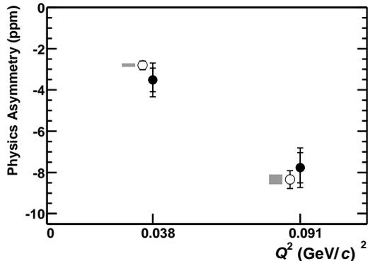
FIG. 2: The physics asymmetries measured in SAMPLE II (updated results) and SAMPLE III are plotted as a function of  $Q^2$  (solid circles). Also plotted (with offset  $Q^2$  for visibility) are the theoretical predictions with the value of  $G_A^e$  taken from Ref. [8], and  $G_M^s = 0.15$  n.m. (open circles). The height of the gray rectangles represents the change in the physics asymmetry corresponding to a 0.6 n.m. change in  $G_M^s$ .
