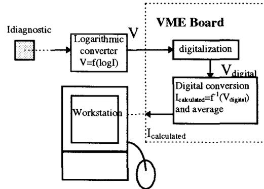
As seen before, the characteristic  $V=f(I)$  isn't linear on the whole scale. We have a non-linearity for low current ( $I < 10pA$ ) and high current ( $I > 100\mu A$ ). The theoretical equation  $V=2 \times \log(I/I_o)$  and the inverse equation ( $I_{calculated} = I_o \times 10^{V/2}$ ) can't be used.
