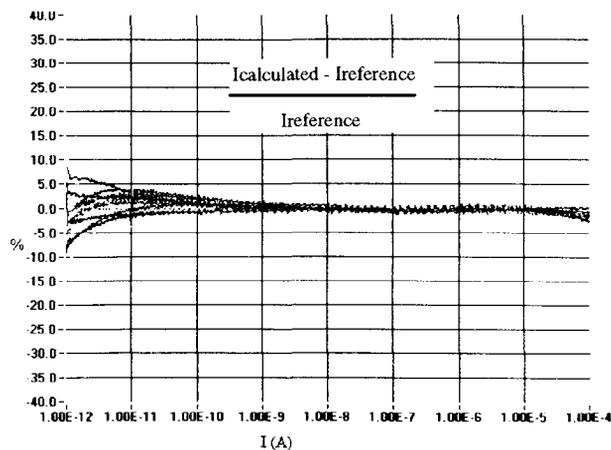
The precision for the low current ( $i < 10^{-10}$  A) decreases because diodes have different characteristics.
