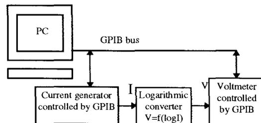
We acquire 1000 measurements of the characteristic  $V=f(I)$ . We choose an average characteristic and a computer program calculates the characteristic  $I=f(V)$  with 4096 points. We use an analog to digital converter with 12 bits precision ( $2^{12}=4096$  values).
