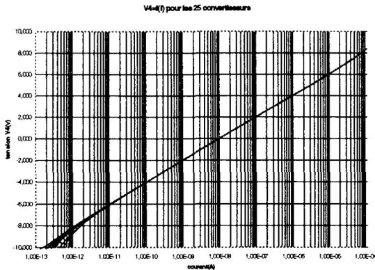
The different converters, for the same room temperature (25°C), have different characteristics for low current. These light differences are due to different values of Is.
