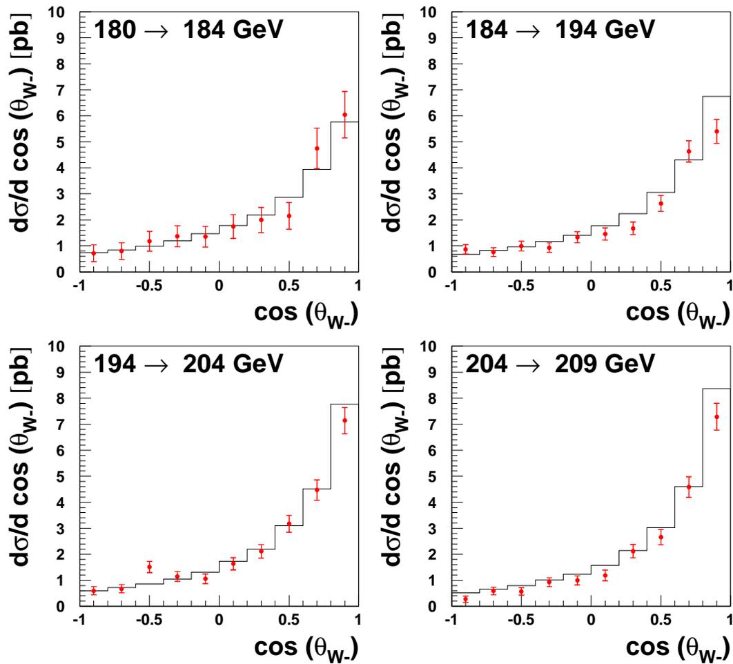
Figure 5:  $W^-$  polar angle differential cross-sections from the  $q\bar{q}e\nu$  and  $q\bar{q}\mu\nu$  channels (detailed definition in the text). The measurements in the four energy bins defined in the text (points) are compared with the expectations (histograms). The systematic contributions are included in the error bars.
