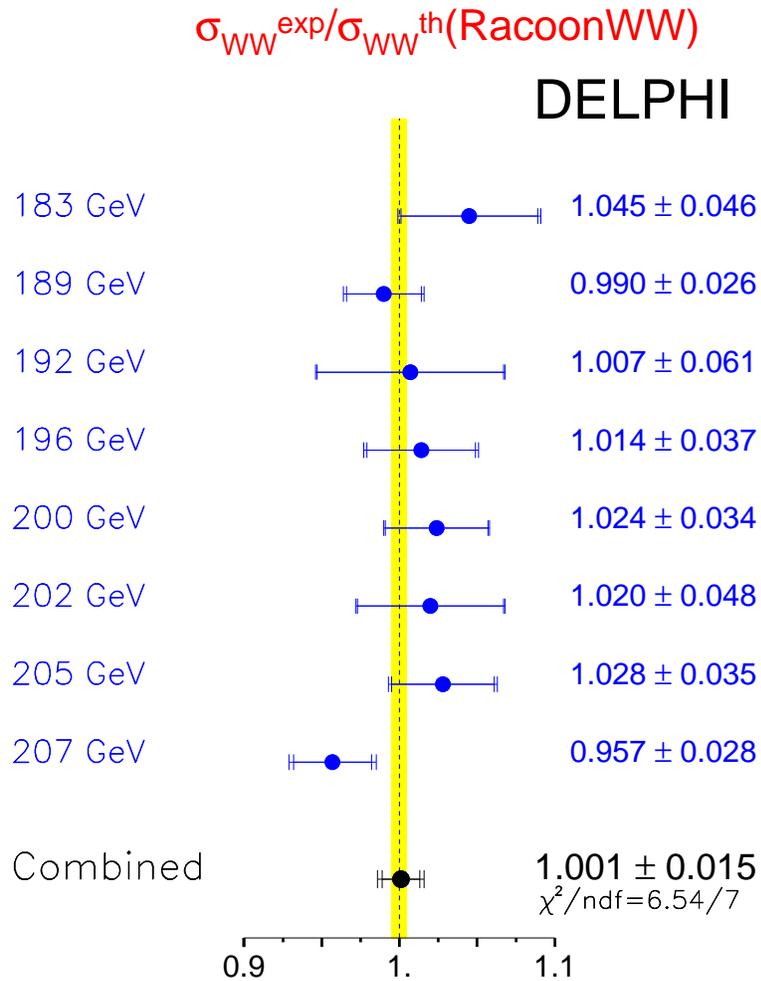
Figure 8: Ratios between measured and predicted CC03 cross-sections with the DELPHI data. The error bars indicate the combined statistical and systematic uncertainties. The energy-combined values are indicated at the bottom. The plot refers to the RACOONWW predictions, where a 0.5% theory error is indicated as a band.
