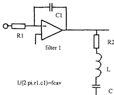
The integrator has a constant  $R1c1$  corresponding to the cavity time constant (1.5KHz) as in the amplitude loop.
