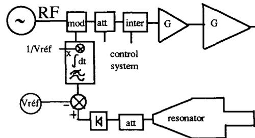
With the choosen control system we plot the gain and phase of the open loop to verify the whole stability.
