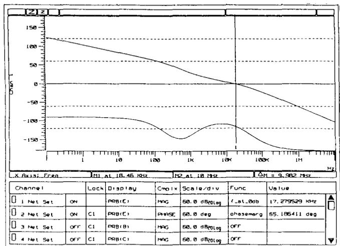
The phase margin is 65° and the frequency is 17 KHz for 0 dB.
