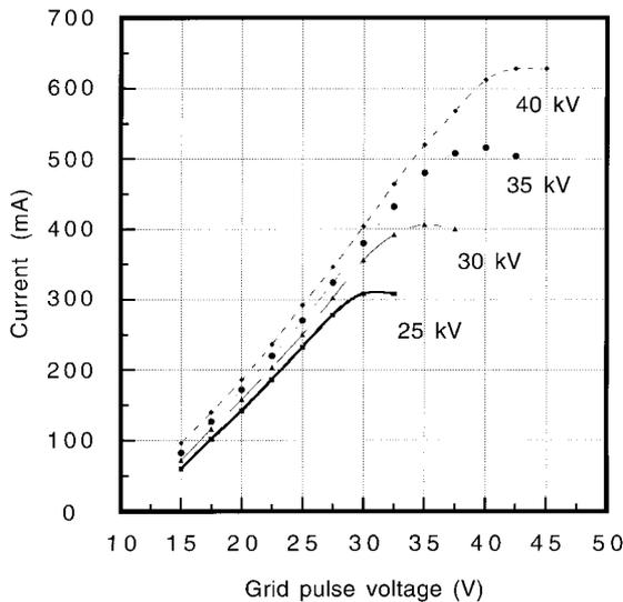
Figure 2. Measured characteristics of the modified gun for varying A-K voltages.
