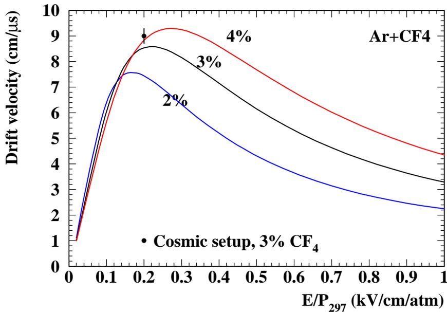
Fig. 2. The drift velocity of electrons as a function of the drift electric field for Ar mixtures with 2, 3 and 4% of CF<sub>4</sub>, as predicted by Magboltz. The data point is the measurement with the cosmic ray setup, with 3% of CF<sub>4</sub>.
