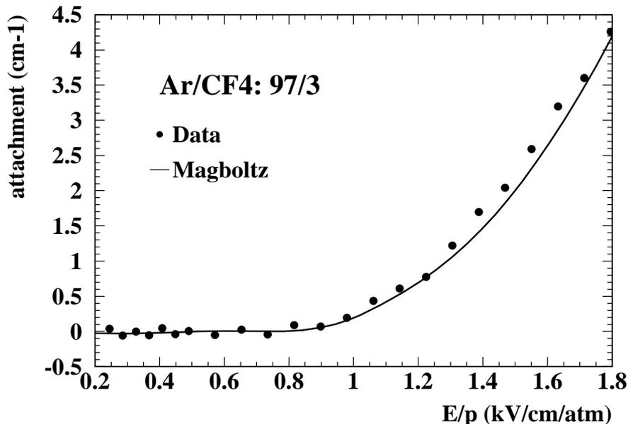
Fig. 4. Attachment coefficient of an Argon (97%)  $\text{CF}_4$  mixture as a function of the electric field. The points are data described in the text and the line is the Magboltz Monte Carlo prediction.
