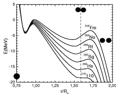
Figure 3. Potential barriers including shell effects for the symmetric fission of  $^{258}\text{Fm}$ ,  $^{260}\text{No}$ ,  $^{260}\text{Rf}$ ,  $^{262}\text{Sg}$ ,  $^{266}\text{Hs}$  and  $^{270}\text{110}$ .
