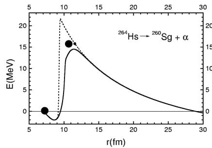
Figure 4. Potential barrier including empirical microscopic corrections against emission of  $\alpha$  from the  $^{264}\text{Hs}$  parent nucleus. The dashed and solid lines correspond respectively to the deformation energy without and with a nuclear proximity energy term.
