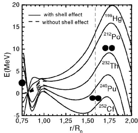
Figure 2. Potential barriers with and without shell effects for the symmetric fission of  $^{198}\text{Hg}$ ,  $^{212}\text{Po}$ ,  $^{232}\text{Th}$ ,  $^{240}\text{Pu}$  and  $^{252}\text{Cf}$  versus the mass center distance.
