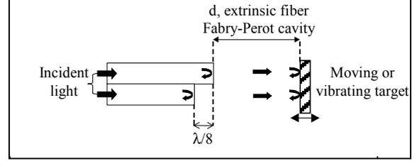
Fig. 2. b) Dual extrinsic Fibre Fabry-Perot interferometer proposed by Claus et al.<sup>8</sup>
