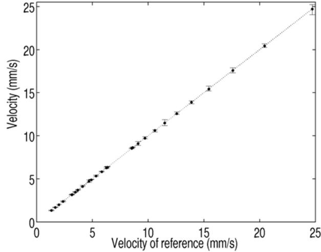
Fig. 10. Comparison of the velocity measurement between a reference device and our sensor with a PZT excitation amplitude of 1,3 V<sub>pp</sub> while a variable frequency.
