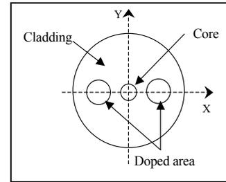
Fig. 6. Cross section of the Panda<sup>TM</sup> fibre
