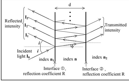
Fig. 1. a) Principle of the Fabry-Perot cavity.
