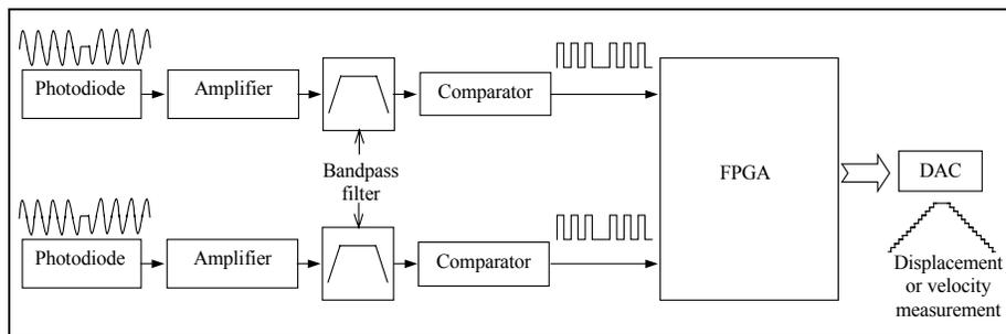
Fig.7. Simplified block diagram of the signal processing.
