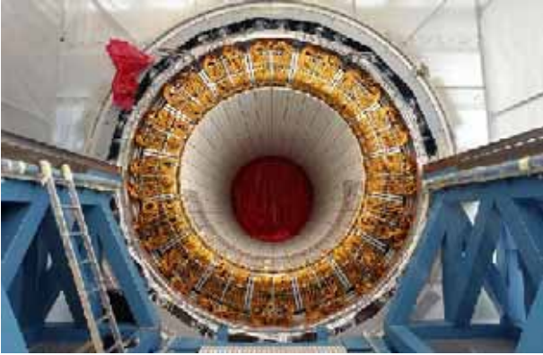
Figure 2. First half barrel inserted inside the ATLAS cryostat
