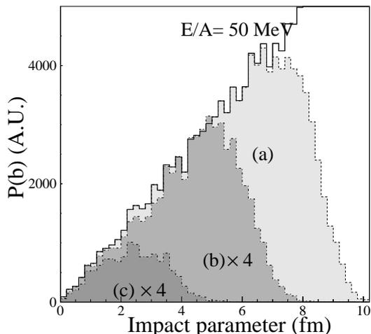
Figure 1: Impact parameter distributions for the reaction  $^{129}\text{Xe}+^{120}\text{Sn}$  at 50 MeV/A as given by the model filtered by the INDRA filter software. Unfilled histogram: all simulated events. Other histograms are labelled according to the selection discussed in the text. Note that, in cases (b) and (c), the distributions have been multiplied by a factor 4
