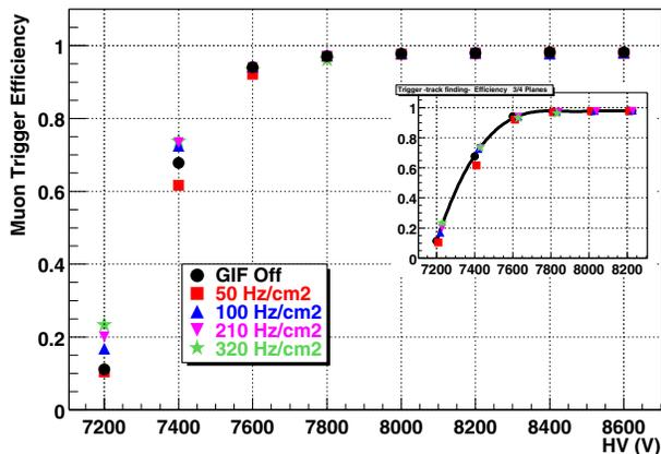
Fig. 2. Efficiency of the muon trigger test experiment with different level of background (created by the  $\gamma$  source of GIF) as a function of the high voltage applied to the RPCs. The efficiency is measured with respect to hodoscopes (scintillators associated with photomultipliers).
