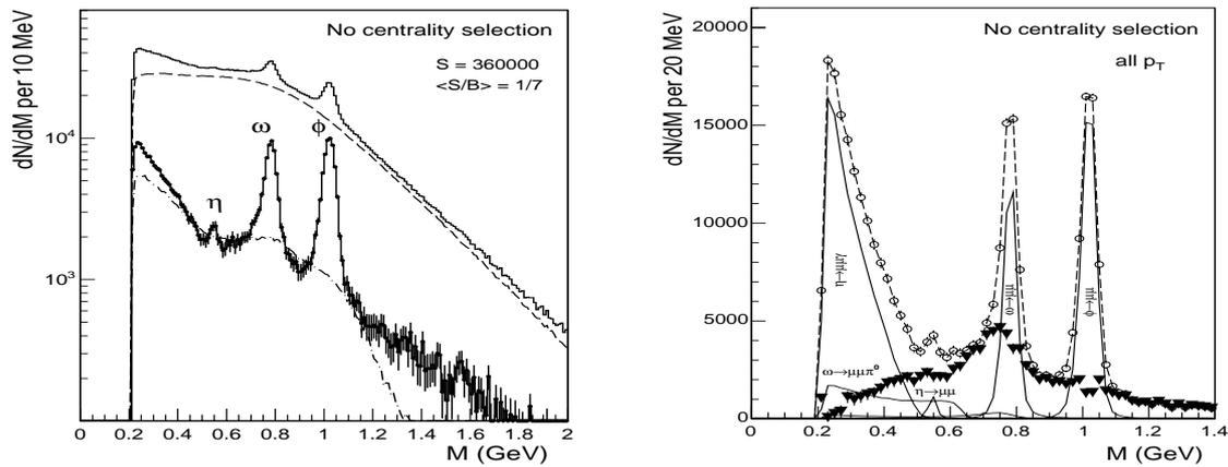
**Figure 2:** Left: Measured opposite-sign dimuon mass spectra (upper line), combinatorial background (dashed), fake matches (dashed-dotted) and extracted signal. Right: Illustration of the isolation procedure: the  $\eta$ ,  $\eta'$ ,  $\omega$  and  $\phi$  contributions (solid lines) are subtracted from the signal spectrum (circles) to give the excess (triangles).
