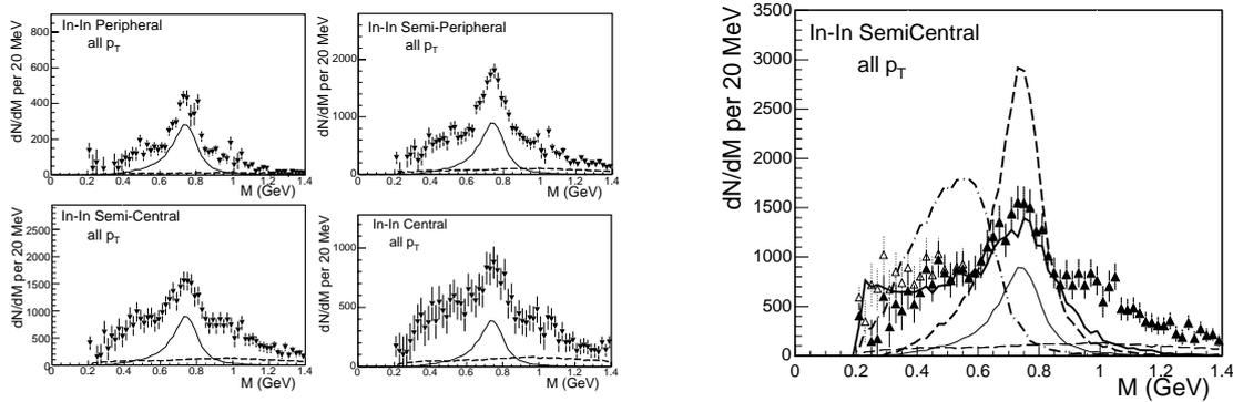
**Figure 3:** Excess dimuon mass spectra; the cocktail  $\rho$  (thin solid) and the level of open charm (thin dashed) are shown for comparison. Left: Centrality dependence. Right: Comparison to model predictions [6], prepared for In-In at  $dN_{ch}/d\eta = 140$ . Unmodified  $\rho$  (dashed), in-medium broadening  $\rho$  (Rapp-Wambach, solid), in-medium dropping  $\rho$  (related to Brown-Rho scaling, dashed-dotted).
