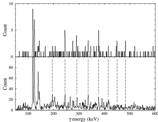
Figure 1. Bottom: Rotational band of  $^{251}\text{Md}$  obtained using  $\gamma$  spectroscopy. The top spectrum shows the results of gates set on the main rotational bands using  $\gamma$ - $\gamma$  coincidences.
