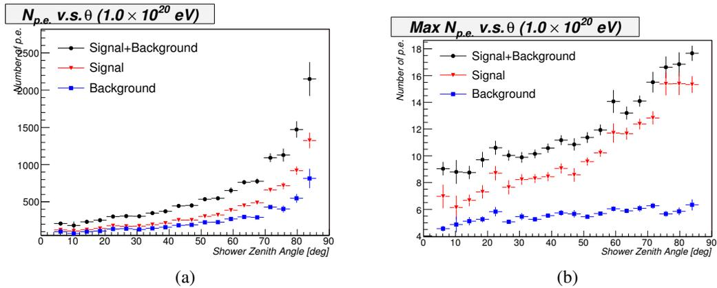
**Figure 3.** (a) Number of counts on the EUSO focal surface generated by  $10^{20}$  eV showers as a function of the shower zenith angle. (b) Number of counts in the most populated pixel on EUSO focal surface as a function of shower zenith angle. EUSO Redbook requirements configuration was used. Background counts are limited to the pixel with signal.
