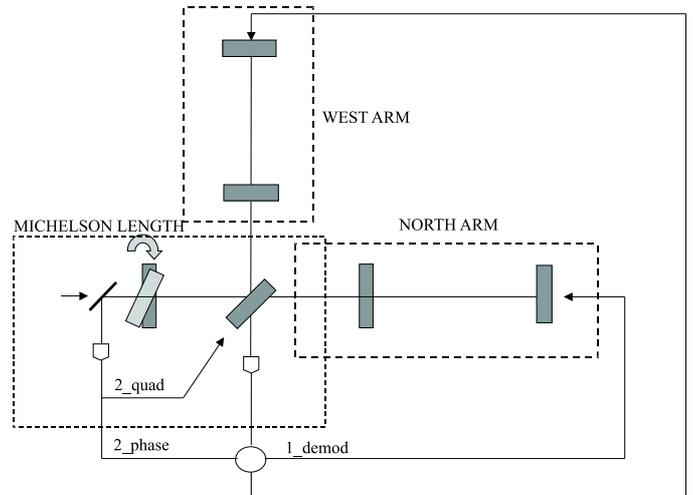
Fig. 6. Linear locking of the recombined ITF: the end photodiodes signals are replaced with the reflected and the output port one, because of noise reasons.
