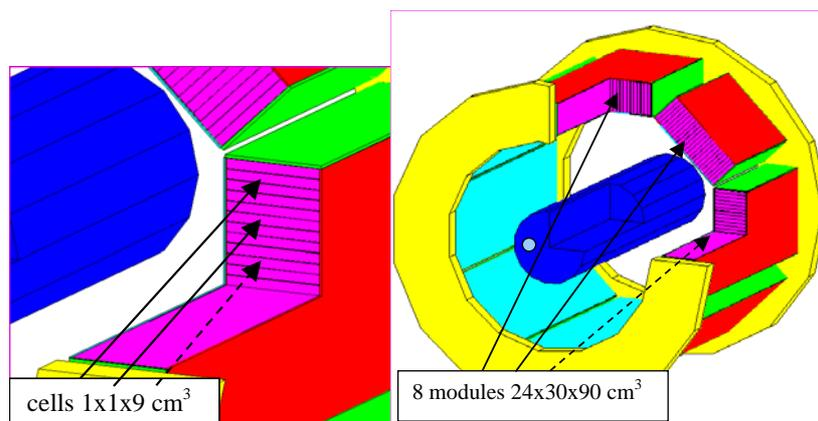
Fig. 1. GEANT3 simulation of a LXe PET camera with a NEMA NU 2-2001 phantom (right) and zoom on individual cells (left). The  $^{18}\text{F}$  source is homogeneously distributed in a 3 mm diameter and 70 cm length cylinder positioned at  $(x=4.5 \text{ cm}, y=0 \text{ cm})$  in the transverse field of view.
