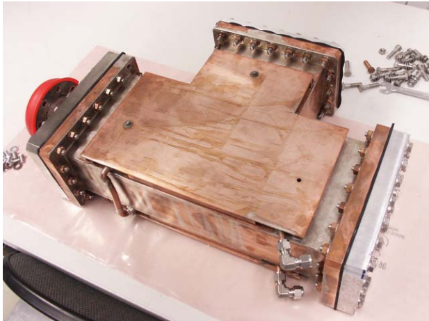
Figure 2: Photograph of the power combiner.
