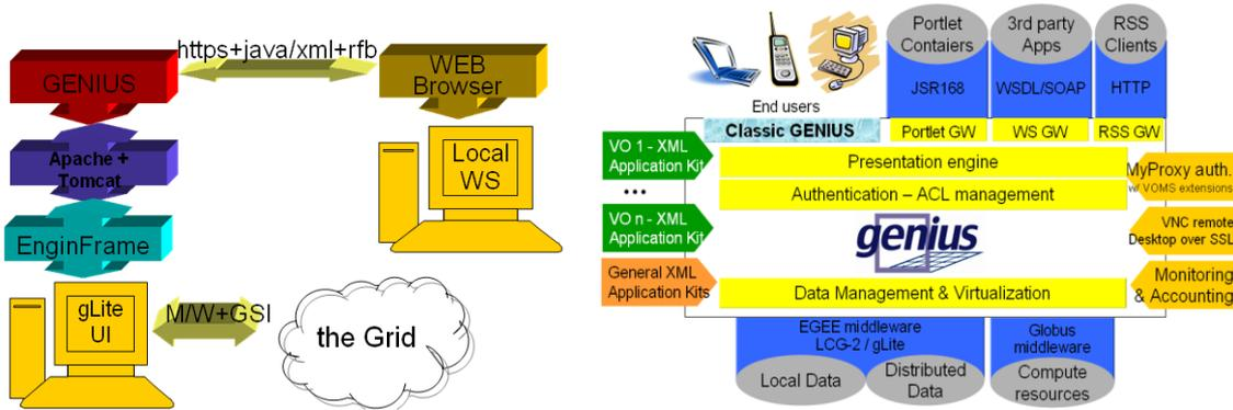
Figure 1: Three-tier architecture of the GENIUS portal
