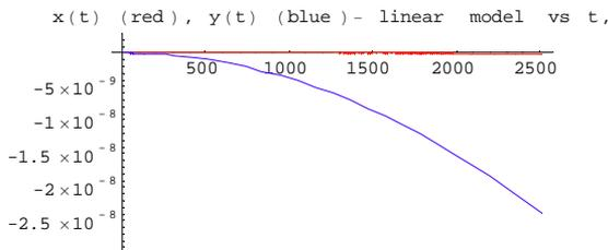
Figure 2. Difference between numerical solution and the simplified model with sine replaced by its argument and cosine by 1. Red is for  $x(t)$ , blue  $y(t)$ . Note change of scale compared to Figure 1.
