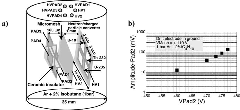
Figure 2. a) Schematic view of the Piccolo-Micromegas detector for neutron flux measurements inside a nuclear reactor. b) Variation of the amplitude of the signal of one PAD of Piccolo-Micromegas detector versus High Voltage (HV) of the PAD for fixed Mesh Voltage at +110 V, the drift cathode in the ground and 1 bar Ar+iC<sub>4</sub>H<sub>10</sub>.
