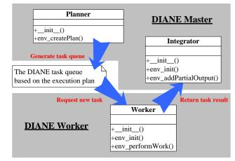
Fig 2 the template of DIANE application plug-ins as well as the cooperation model between the three major objects: Planner, Worker and Integrator.
