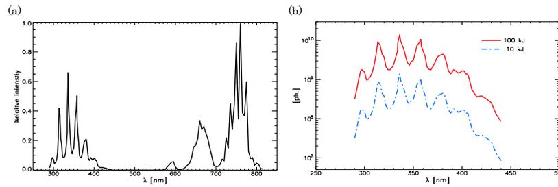
**Figure 2.** (a) Relative optical intensity spectrum of sprites [3]. (b) Estimated photon number spectrum of sprites in the range of 290–440 nm at the entrance of the EUSO telescope at ISS. Note that the atmospheric transmission is supposed to be 1.0
