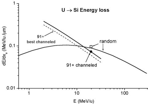
Figure 4: Expected evolution of the energy loss for channelled  $\text{U}^{91+}$  ions in the  $\langle 110 \rangle$  axis of silicon. The experimental data (circle: most probable energy loss in channelling, square: loss for random orientation) are taken from ref. [16]. The random energy loss curve corresponds to SRIM calculations [21]. The dashed curve corresponds to the loss experienced by the best-channelled ions.
