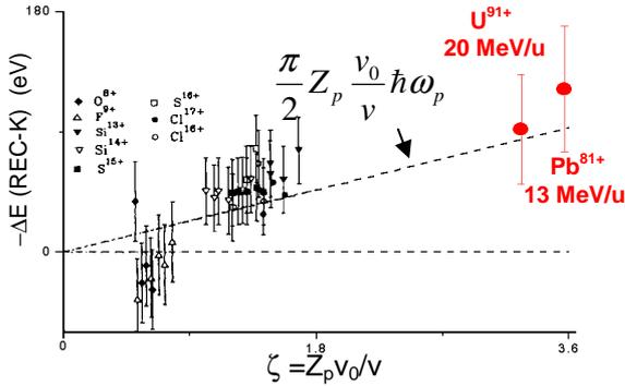
Figure 3: K- and L-REC line shift due to the wake potential induced by channelled heavy ions in silicon  $\langle 110 \rangle$ . The data for  $\zeta < 1.8$  are from Tribedi et al. [20]. The dashed line corresponds to linear response theory calculations [19] for a free electron gas of density  $0.2 \text{ e}^{-}/\text{\AA}^3$  ( $\hbar\omega_p = 16.6 \text{ eV}$ ). The data for  $\text{U}^{91+}$  and  $\text{Pb}^{81+}$  ions are from Testa et al. [18].
