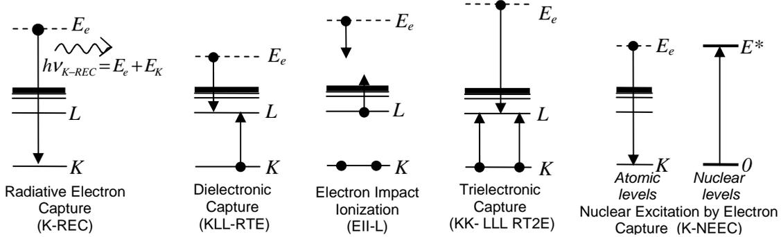
Figure 1: Schematic description, in the projectile frame, of charge exchange processes observable in highly charged ion channelling conditions.  $E_e$  represents the kinetic energy of a target electron.
