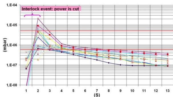
Figure 3: Examples of vacuum recovery after an interlock event.
