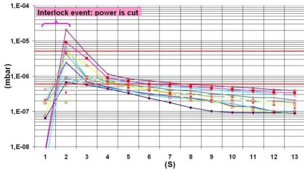
Figure 3: Examples of vacuum recovery after an interlock event.
