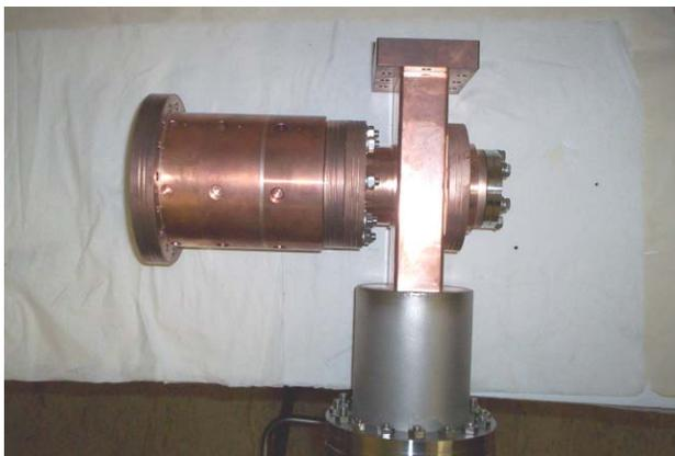
Figure 7: The completed ALPHA-X photo-injector.
