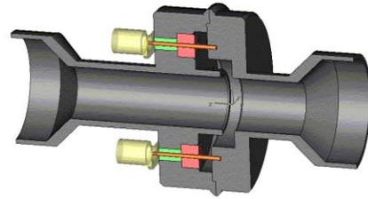
Figure 5 : BPM for the probe beam linac.
