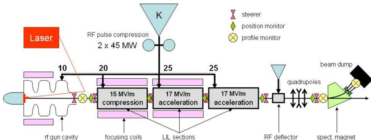
Figure 1: Schematic layout of the probe beam linac (Califes).
