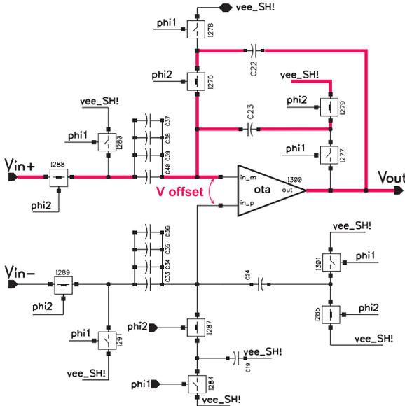
Figure 3: Sample and Hold Amplifier (SHA) scheme.
