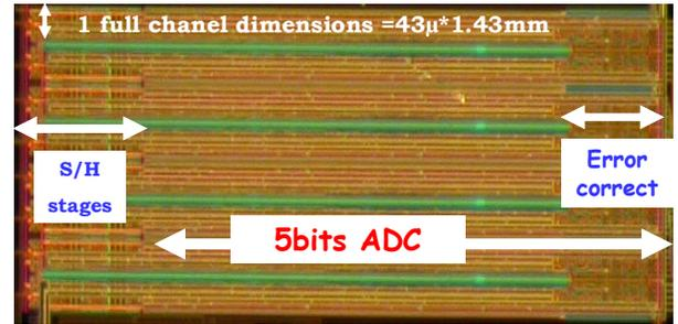
Figure 11: Layout of a prototype with 8 channel ADC.
