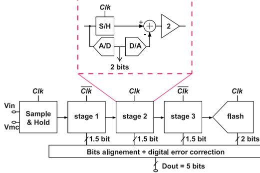
Figure 2: General block diagram of a pipelined converter.
