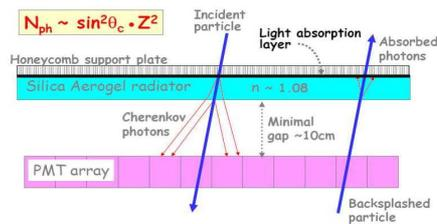
Fig. 1. *Scheme of the Cherenkov imager principle.*
