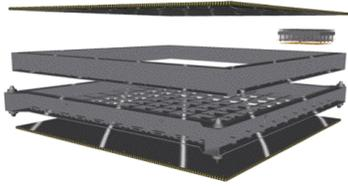
Fig. 2. Exploded view of the CHERCAM mechanical structure. The detector plane is arranged in  $5 \times 5$  blocks of 64 PMT. Each block is divided into 4 modules of  $4 \times 4$  PMT, each being read out by a single 16-channel FE electronics circuit.
