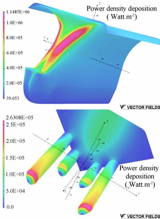
Figure 5: Power density deposition on vane and rods.
