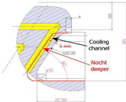
Figure 2: IPHI vane end profile and cooling channel.
