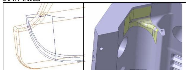
Figure 1: IPHI 6-meter section vane end profile modification.
