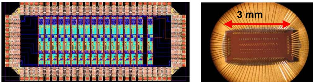
Figure 2: LPNHE front end layout: 16 + 1 channels (left side), and chip delivered by the foundry (right side)
