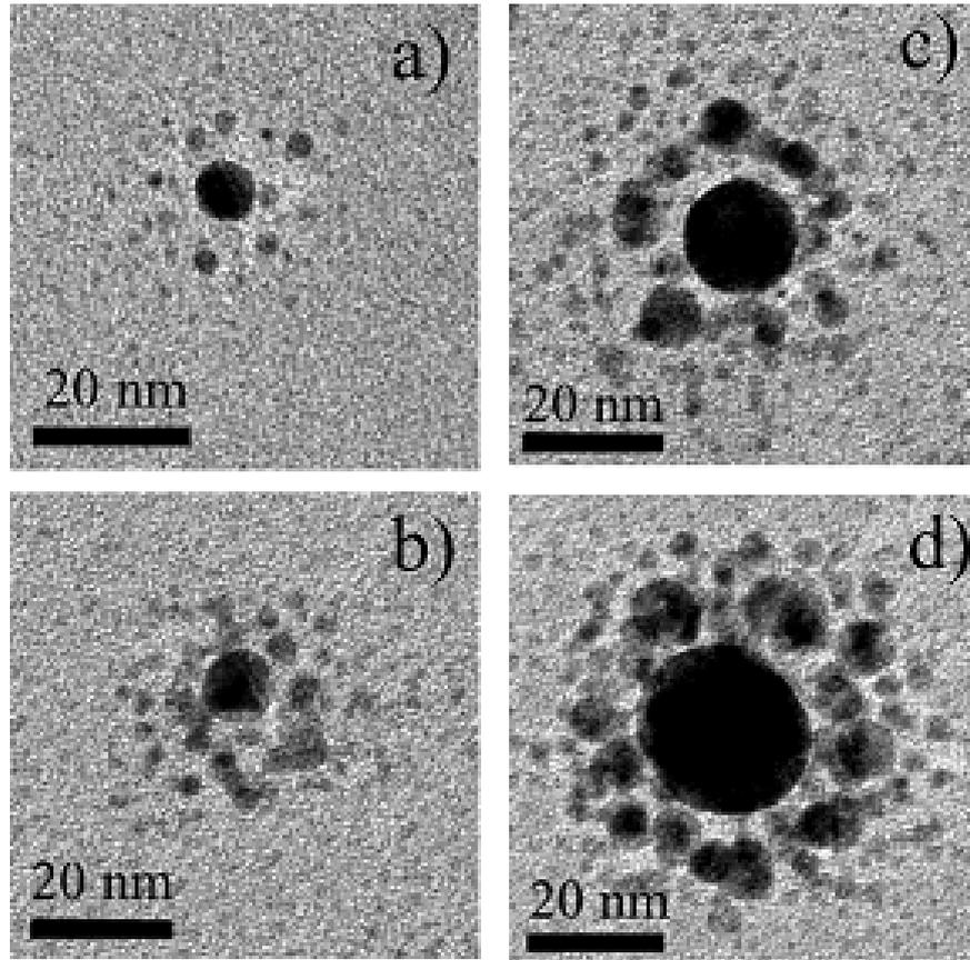
FIG. 2: TEM micrograph of NCs with different sizes irradiated at a fluence of  $1.5 \times 10^{16} \text{ cm}^{-2}$  with 4 MeV Au ions at room temperature. a) 5.8 nm, b) 8.7 nm, c) 16.7 nm and d) 25.1 nm.
