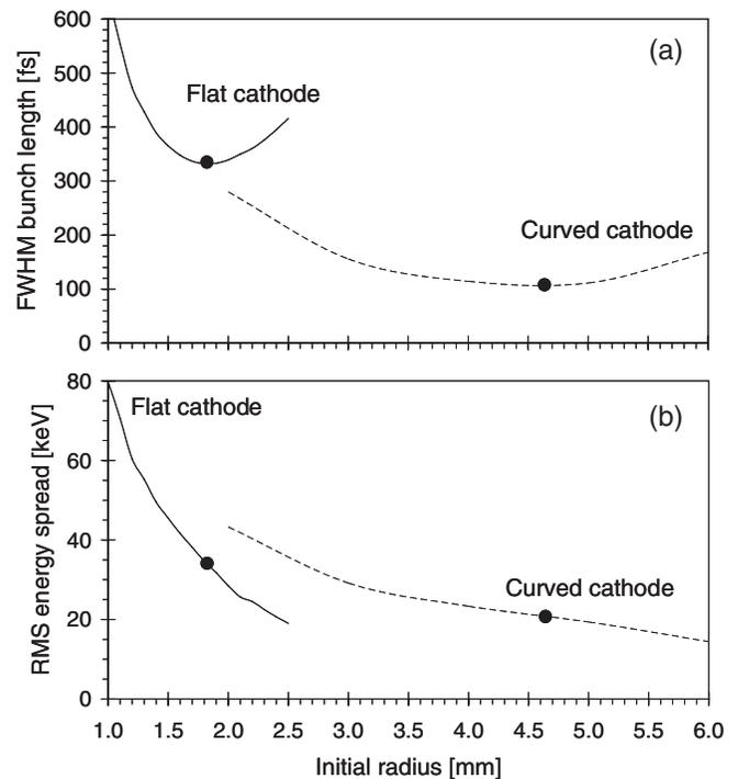
FIG. 2. (a) Bunch length of a 10 pC electron bunch at the entrance of the plasma channel, at  $z = 1.85$  mm, as function of initial radius. (b) Corresponding energy spread. The initial radii resulting in minimum bunch lengths are indicated by dots.
