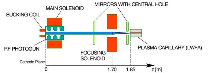
FIG. 1. (Color) Schematic of the Alpha-X setup.
