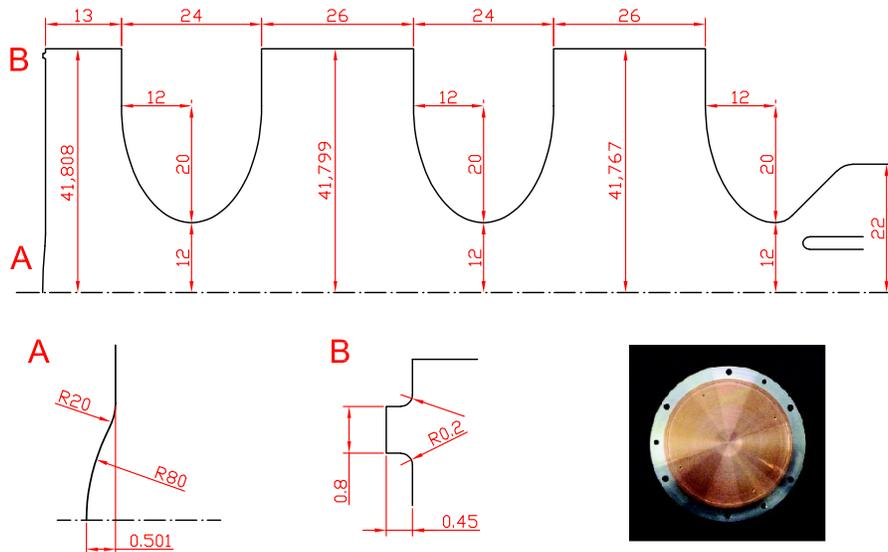
FIG. 6. (Color) Simplified inner dimensions of the rf-photogun with curved cathode. Detail A shows the dimple to compensate for path-length differences on a 5:1 aspect ratio, detail B shows the compensation groove with 1:1 aspect ratio.
