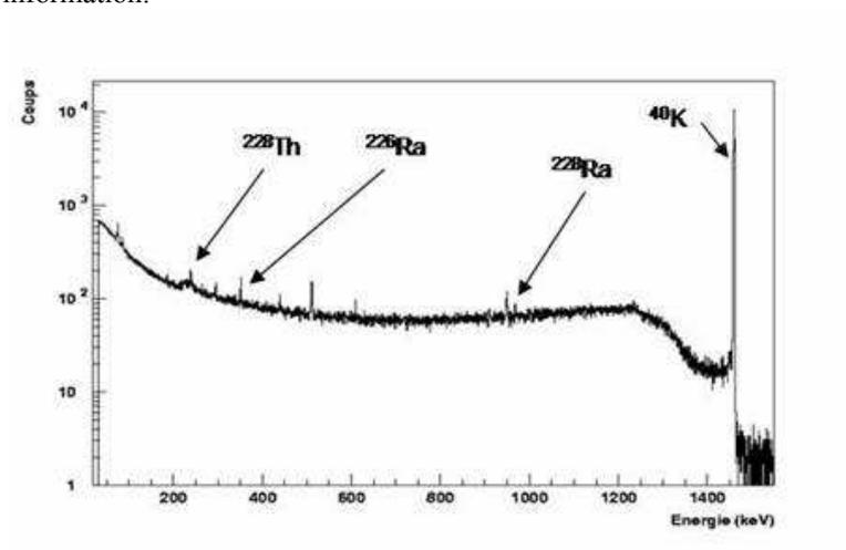
FIGURE 4. Gamma spectrum of a sample of prunes from Agen.
