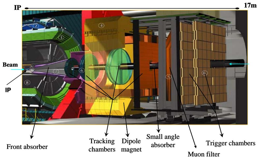
**Figure 1** : Layout of the ALICE muon spectrometer.
