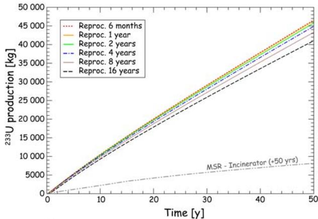
Fig. 7. <sup>233</sup>U production for various Pu-operated MSR fuel reprocessing times and for the MSR-incinerator
