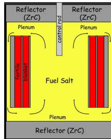
Fig. 2. Vertical section of the fast TMSR core
