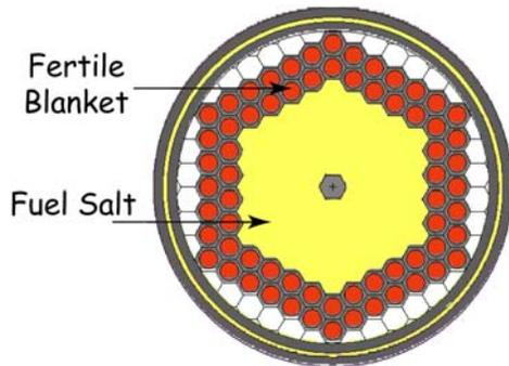
Fig. 3. Horizontal section of the fast TMSR core
