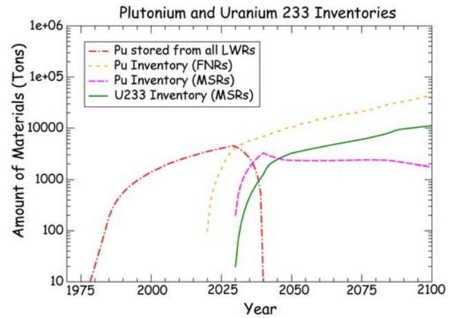
Fig. 11. Inventories in Plutonium and <sup>233</sup>U for two deployment scenarios: with LWRs and FNRs, and with LWRs, MSR<sub>s</sub> started with Pu and TMSRs
