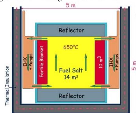
Fig.1. To scale vertical representation of the TMSR, including pumps and heat exchangers (IHx)
