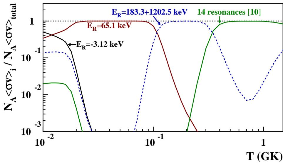
FIG. 8: (Color online) Ratios of individual reaction rate contributions to the total modal rate for the  $^{17}\text{O}(p,\alpha)^{14}\text{N}$  reaction. The unlabelled solid and dashed lines below 0.02 GK correspond to tail contributions of the resonances at 0.557+0.677 MeV and 1.202 MeV, respectively (see text).
