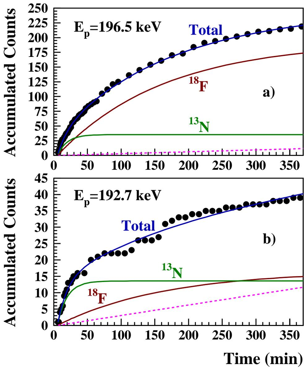
FIG. 7: (Color online) Measured  $\beta^+$  activities of two  $^{17}\text{O}$ -implanted targets irradiated at (a)  $E_p^{\text{lab}}=196.5$  keV (on-resonance) and (b)  $E_p^{\text{lab}}=192.7$  keV (off-resonance). The time origin corresponds to the stopping of the proton irradiation. Also shown are the fitted  $^{18}\text{F}$  and  $^{13}\text{N}$  decay curves (solid lines) and the measured background radiation (dashed lines).
