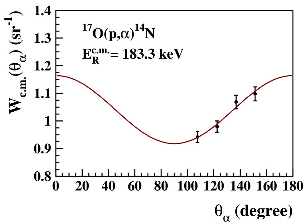
FIG. 5: (Color online) Angular distribution (center of mass) for the  $^{17}\text{O}(p,\alpha)^{14}\text{N}$  resonance at  $E_{\text{c.m.}}=183.3 \text{ keV}$ . The solid line shows a Legendre-polynomial fit to the data points,  $W_{\text{c.m.}}(\theta_{\alpha}) = 1 + a_2 P_2(\cos\theta_{\alpha})$ , which yields  $a_2=0.16\pm 0.03$ .
