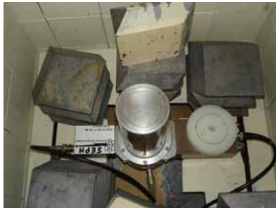
Fig. 11: The detector with its Pb shielding
