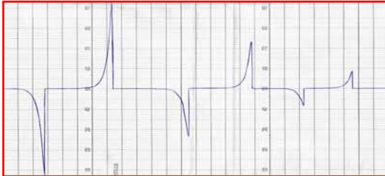
**Fig. 14: Transient response of a PICMA type actuator to various steep preload variation  $\Delta F = \pm n \times 150 \text{ N}$  ( $n=1, 2, 3$ ) at  $T=4.2 \text{ K}$ .**
