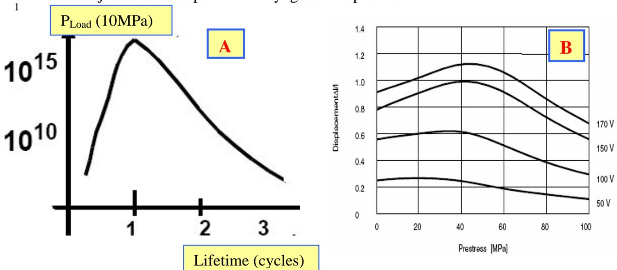
**Fig. 1: A) Sketch of lifetime versus preloading pressure, B) Displacement versus preloading pressure at different voltages (R. Binding et al., see ref. 7).**
