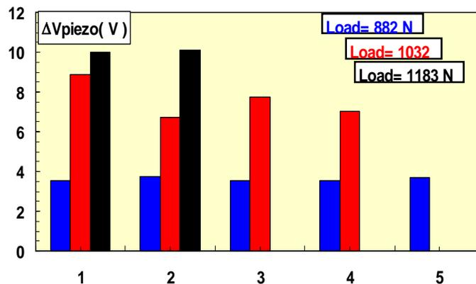
**Fig. 15: Histogram of the peak voltage recorded during transient response of the actuator to various steep preload variation  $\Delta F = \pm n \times 150 \text{ N}$  ( $n=1, 2, 3$ ) at  $T=4.2 \text{ K}$ .**
