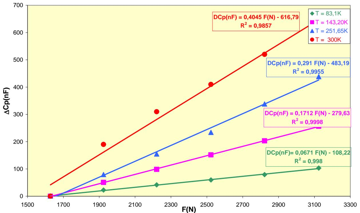
**Fig. 11: Capacitance versus preload for T in the range 83K -300K**
