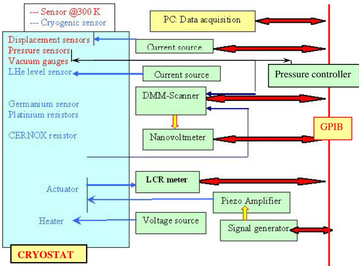
**Fig. 7: Block diagram of the data acquisition system**
