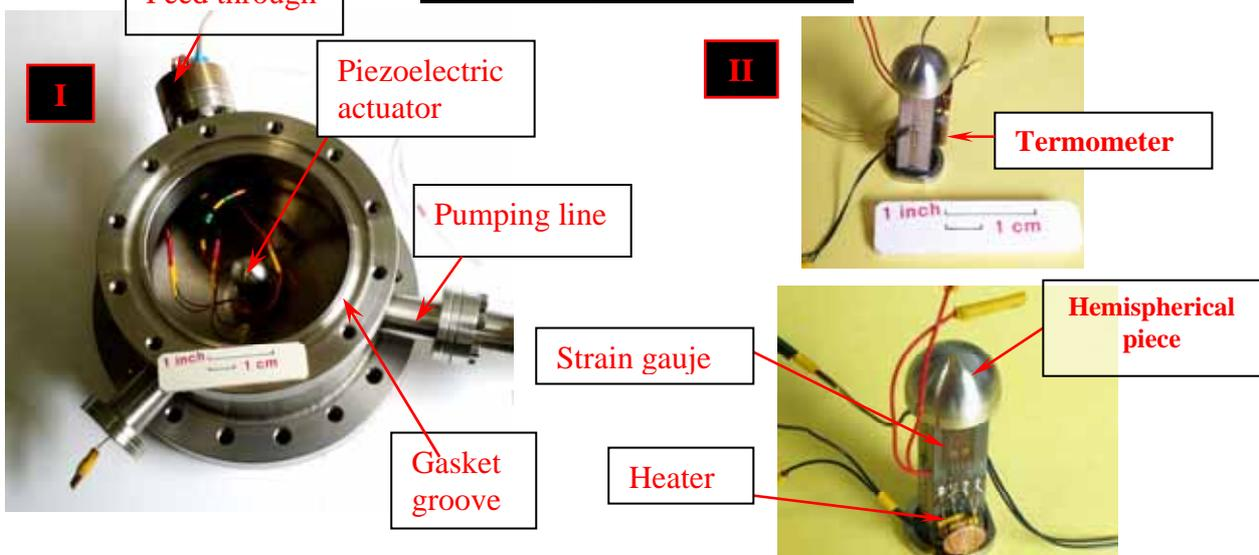
**Fig. 4b: I) Test-cell with piezoelectric actuator during preparation, II) Piezoelectric actuators equipped with heater and a calibrated thermometer**
