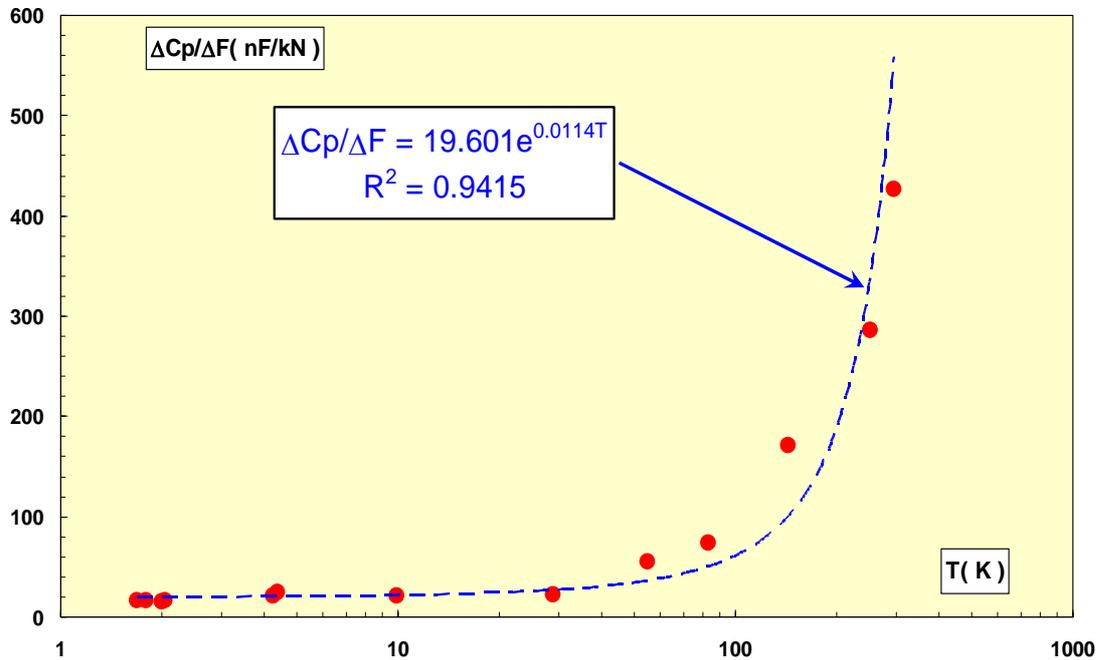
**Fig. 12: Sensitivity to preloading versus temperature**
