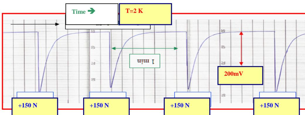
**Fig. 13: Transient response of a PICMA type actuator to a steep preload variation  $\Delta F=150$  N at  $T= 2$  K.**
