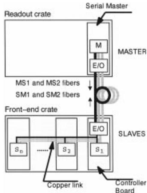
Fig. 2. Architecture of the serial communication system.
