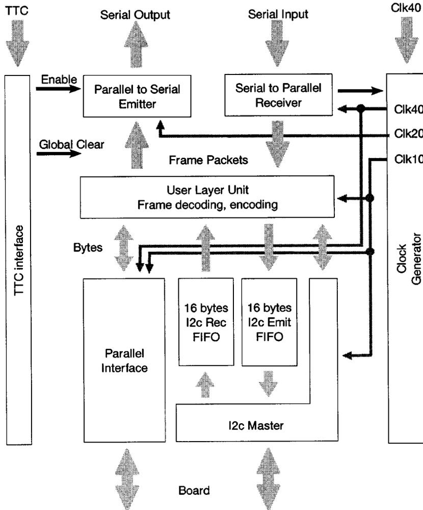
Fig. 7. Functional diagram of the SPAC slave.
