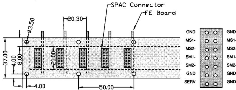
Fig. 6. Schematics of the SPAC copper bus.
