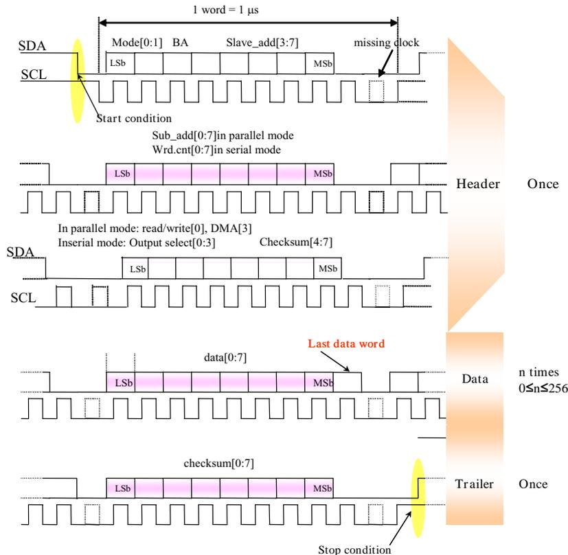
The frame is composed of a fixed size header, a variable size data block, and a fixed size trailer.
