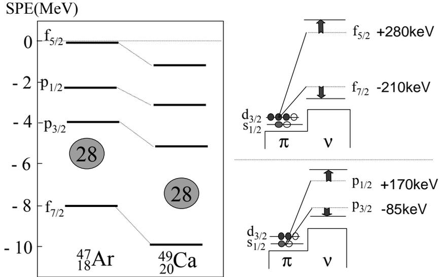
Fig. 2. Left : Neutron single particle energies (SPE) of the  $fp$  orbitals for the  $^{47}_{18}\text{Ar}_{29}$  and  $^{49}_{20}\text{Ca}_{29}$  nuclei. Right : Schematic view of the proton-neutron interactions involved to change the  $f$  (top) and  $p$  (bottom) SO splittings.
