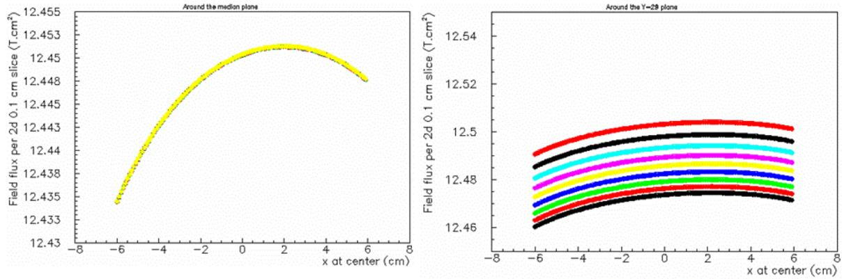
Figure 8: magnetic flux determined in a 1 mm wide spire as a function of the transverse position  $x^{\text{center}}$  for 9 vertical planes equally spaced by 0.5 mm above and below the median plane (left) and the plane  $Y=+29$  mm (right). Each curve represents a vertical plane, the lowest flux corresponding to the lowest value of  $y$ . All 9 curves around the median plane are indistinguishable.
