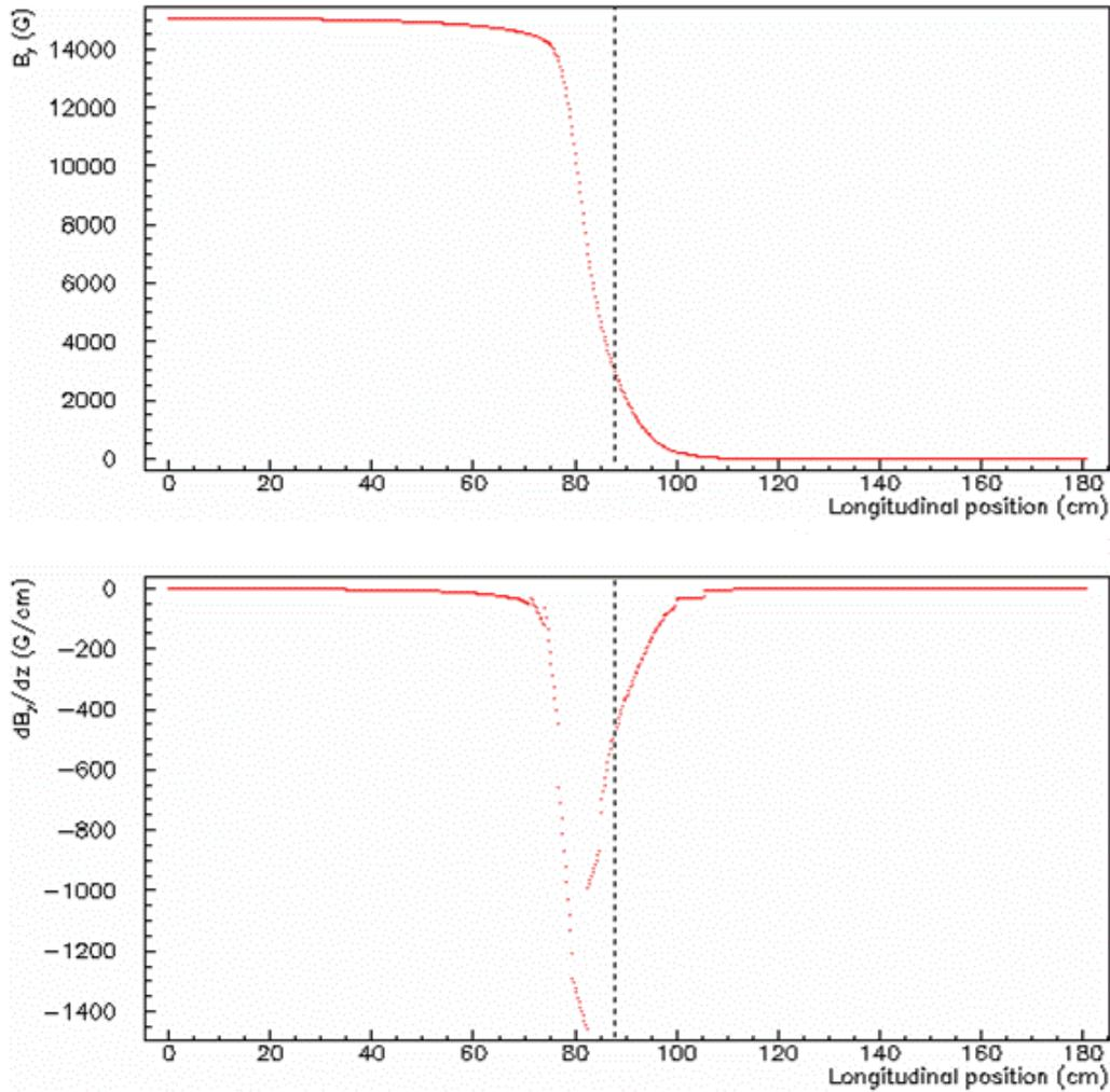
Figure 3: Vertical component of the magnetic field  $B_y$  (top) and its first derivative  $dB_y/dz$  (bottom) as a function of the longitudinal position  $z$  along the central trajectory along the  $z$  axis ( $x=y=0$ ). The dashed line represents the edge of the magnet.
