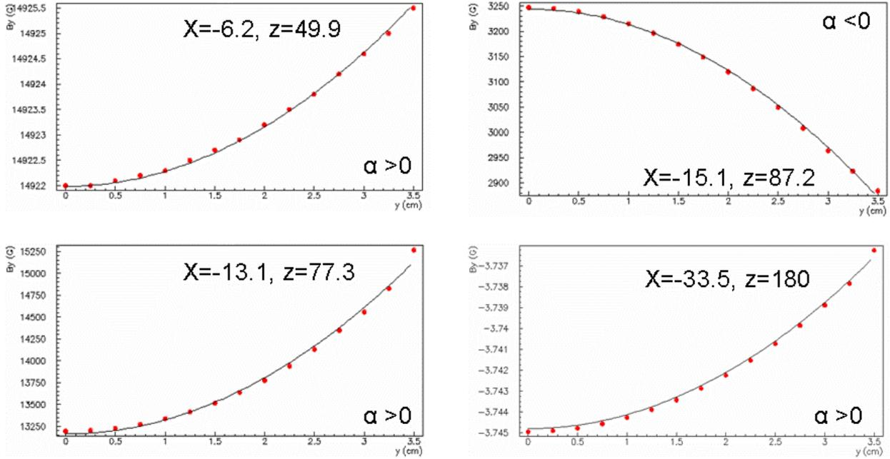
Figure 4: Magnetic field as a function of the vertical coordinate  $y$  for given  $x$  and  $z$  coordinates. Superposed to the data is a parabolic fit (see eq. 5). The parabolic coefficient  $\alpha$  is positive except in a  $\sim 5$  cm long region around the edge of the magnet.
