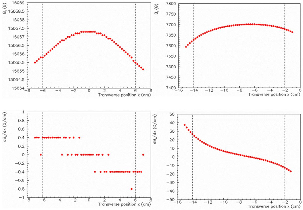
Figure 11: Vertical component of the magnetic field  $B_y$  (top) and its first derivative  $dB_y/dx$  (bottom) as a function of the vertical position  $x$  along the  $x$  axis ( $y=z=0$ ) of the magnet (left) and at the intersection of the median plane and the plane of the magnet edge ( $y=0, z=82$  cm). The dashed line represents the good field region. The discrete aspect of the lower left plot is an artifact of the calculus resolution as  $dB_y/dx$  is very small at the magnet center.
