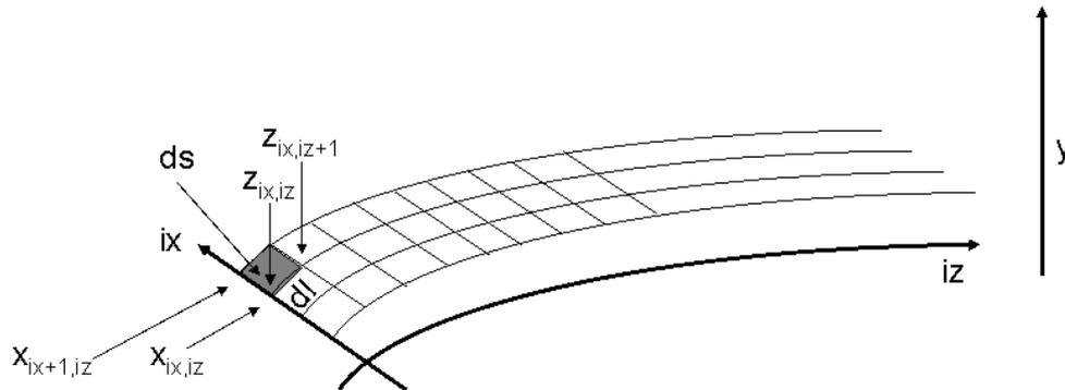
Figure 2: schematics of the notation used for the magnetic field flux calculation. Each data point of the mesh for each vertical plane ( $y$ ) is labelled with an index  $iz$  running along a given trajectory and an index  $ix$  corresponding to the transverse location of the trajectory.
