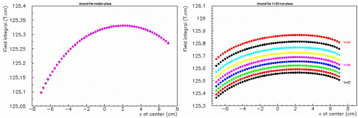
Figure 5: Integral of the magnetic field along a trajectory as a function of the transverse coordinate  $x$ . The 9 different curves on each plot correspond to different vertical planes equally spaced by 0.5 mm above and below the median plane (left) and the  $Y=+29$  mm plane (right). All 9 curves around the median plane are indistinguishable.
