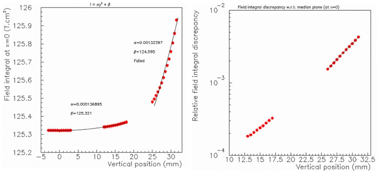
Figure 7: left: Field integrals determined for  $x=0$  as a function of the vertical position  $y$ . Superimposed is a fit assuming a parabolic behavior; right: relative discrepancy between the field integral at a given  $y$  and at  $y=0$  (log scale). Superimposed is a fit assuming an exponential behavior.
