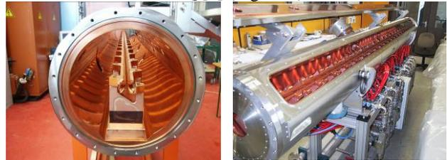
Figure 2: Left: SARAF CW RFQ - 3 MeV 4mA D<sup>+</sup>, 175MHz; right: indust. 4-rod CW RFQ 176 MHz/220kW.
