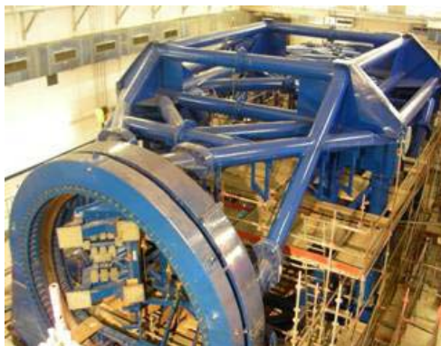
Fig. 7: Photo of the HIT Heidelberg gantry, the total rotating weight is \approx 600 tons, the weight of the last 90^\circ bending magnet is \approx 60 tons.
