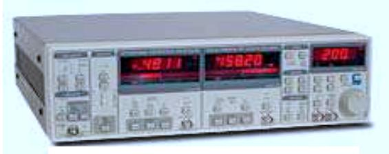
Figure 4: Lock-in Amplifier “SR844”
