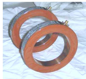
Figure 3: Picture of 2 Fast Current Transformers BERGOZ FCT-082-10:1-WB
