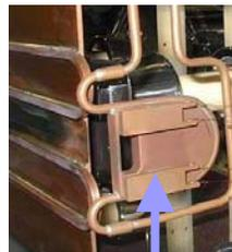
Beam-loss diagnostic inside cyclotron
