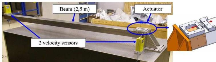
Figure 4: The built mock-up which has similar geometry to the final focus quadrupole
