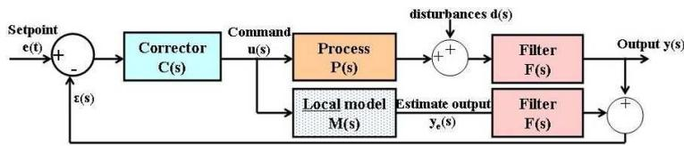
Figure 7: Adaptation of a classic command with internal model control
