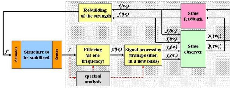
Figure 3: The initial developed algorithm for active compensation
