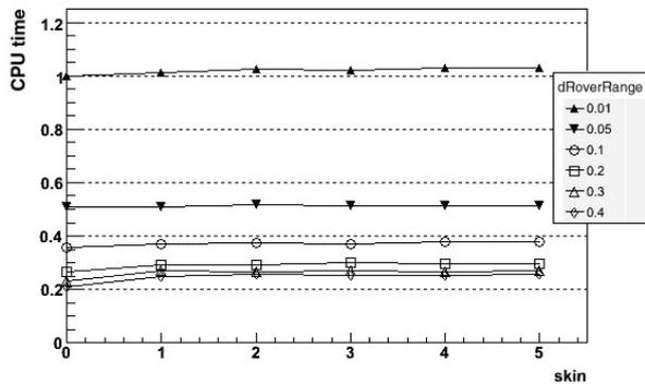
**Figure 8** : Computation time (CPU time) Relative CPU time required for different values of the *skin* and *dRoverRange* parameters. Runs simulated  $10^6$  electrons crossing the cavity normalized to the time for the simulation with parameters (*skin*=0, *dRoverRange*=0.01): about 350 s on Intel 2.66 GHz processor (Woodcrest 5150)
