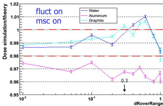
**Figure 7** : response of the cavity with ionization chamber made of different materials
