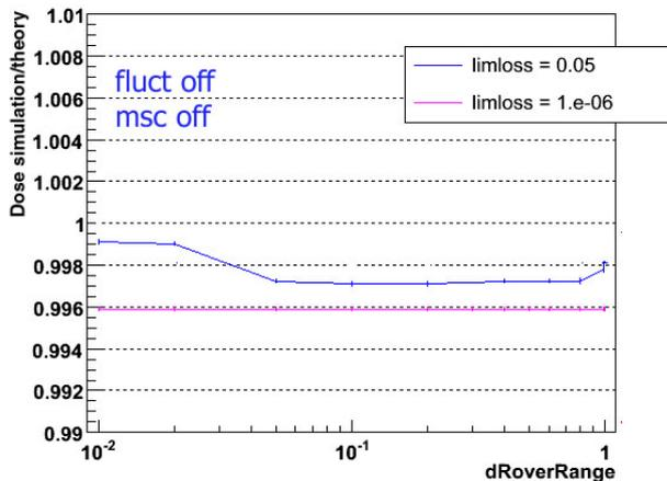
**Figure 3** : response of the cavity (simulated dose deposition divided by the theoretical dose) versus the step limitation parameter  $dRoverRange$
